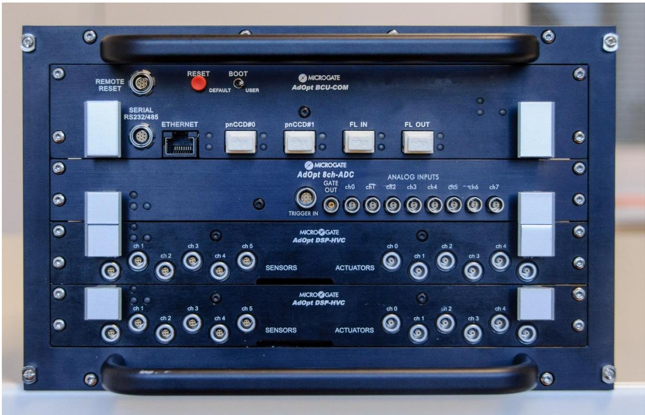
Figure 1 - LGS BCU integrated mini-crate
