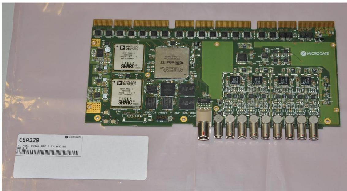
**Figure 4 – The new DSP-ADC 8ch board**
