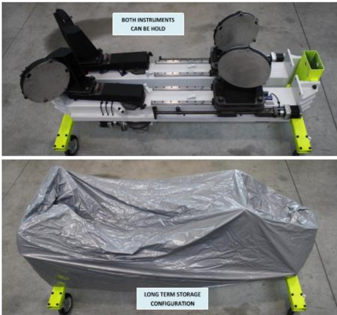
Figure 3. Image of the storage stand with the 2 dichroic mounts mounted on it and the dust cover.
