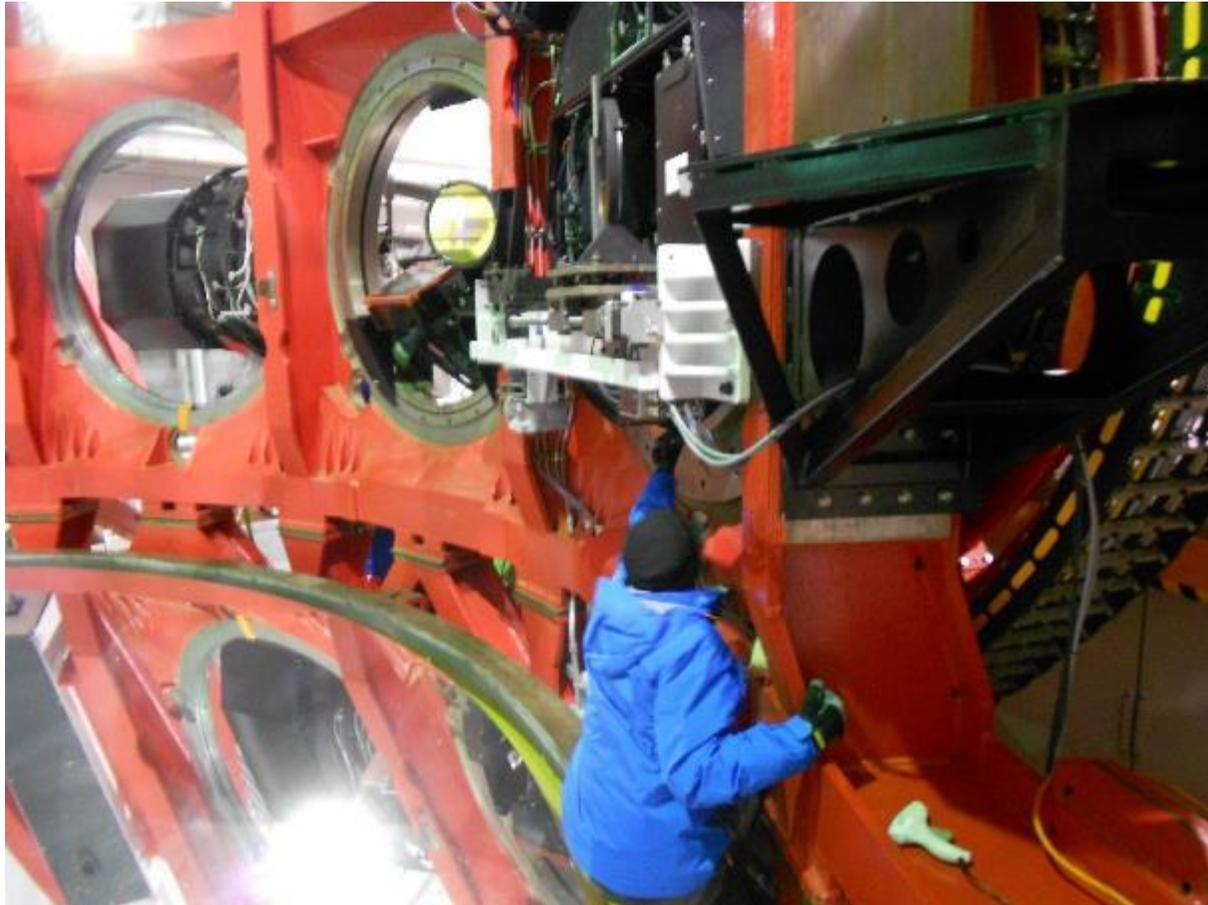
Corner cube and nest glued to rotator flange.
