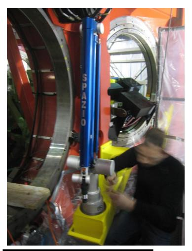
The SPAZIO arm is bolted to the support arm. A reference system centered at the intersection between the rotator axis and the rotator flange is acquired (below, 11.00AM, 2.32)
