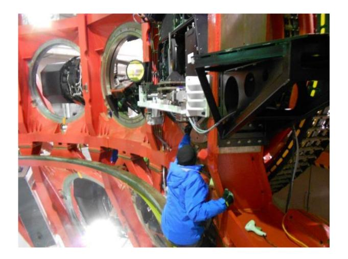
Corner cube and nest glued to rotator flange. Rotator moved and circle fitted to identifiy the axis.
