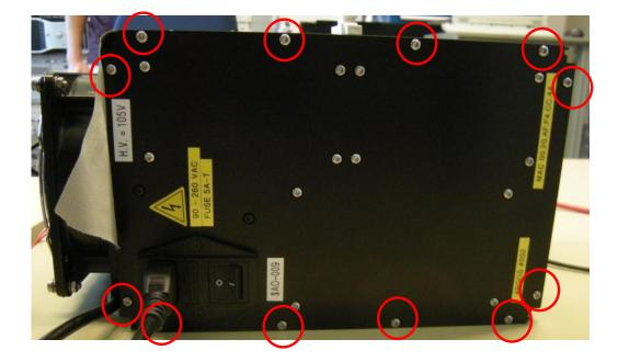
3. Carefully extract the rear panel so that the power supply unit mounted on its internal side becomes accessible.
