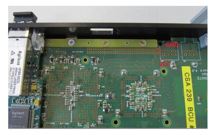
5. Adjust the Power Supply Voltage to read 3.4V on the testpoint described in 4.
