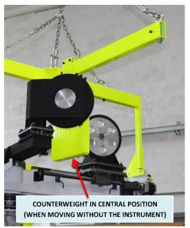
4. Remove the four M14 Allen screws to free the *Handling Device* and remove it.
