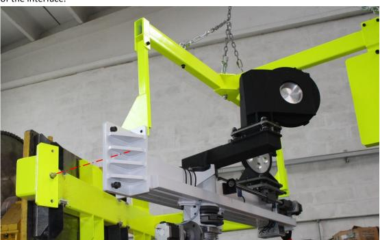
2. Slip the instrument on the *Reference Pins* and fasten the four M18 Allen screws.
