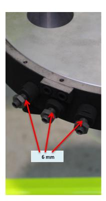
17. Insert from the back of the mounting the Mirror-Lifting tool and screw it about 6 turns
