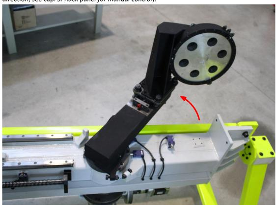
13. Turn the wheel of the Service Stand counterclockwise to make the unit roll of 90°
