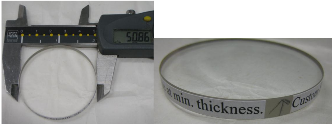
Figure 13. Picture of the 2nd element of the EW. The arrow visible on the right picture marks the thinner edge of the window.
