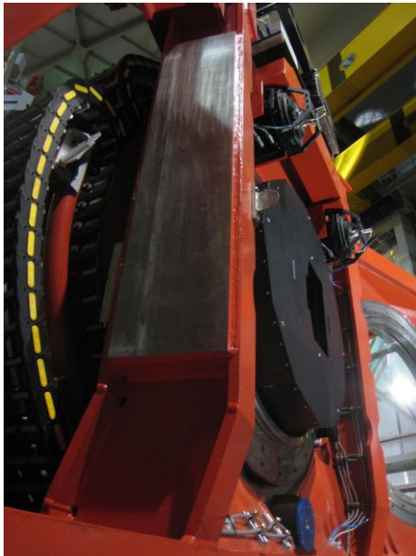
Figure 6 The machined interface on which the measuring support has to be bolted
