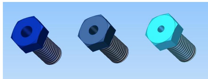
Figure 12 A set of drilled bolts with various diameter of the hole to match the drill tip will be used
