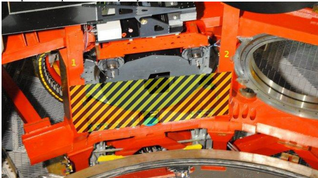
Figure 1 AGW unit at the Lucifer focal station. Area occupied by the dichroic. Beams 1 and 2 indicated
