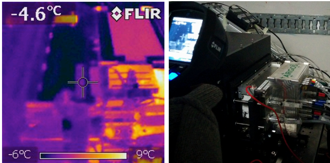
Figure 14 WFS Camera housing is well insulated: the housing surface temperature is -5C, the same temperature of the LGSW enclosure. The measurement has been acquired on the white label that is the only area of the camera surface presenting high emissivity.
