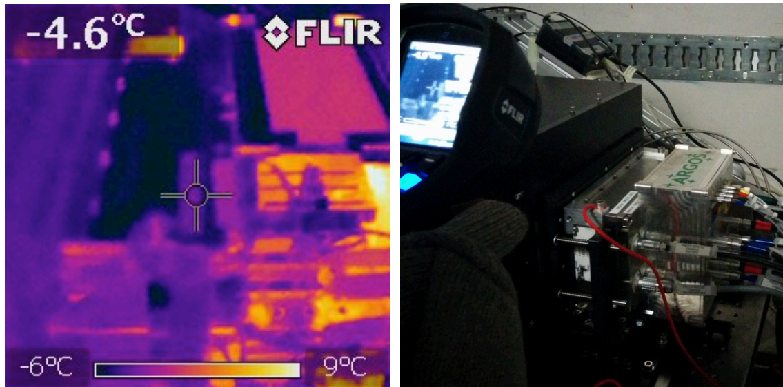
Figure 19 WFS Camera housing is well insulated: the housing surface temperature is -5C, the same temperature of the LGSW enclosure. The measurement has been acquired on the white label that is the only area of the camera surface presenting high emissivity.
