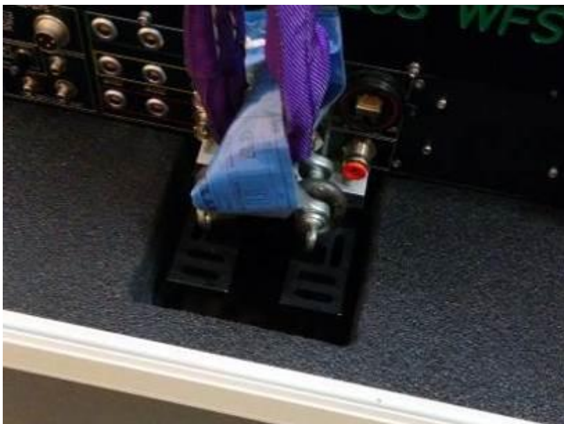
Figura 1. Detail on one of the LGSW lifting pads when it is connected to the lifting frame.
