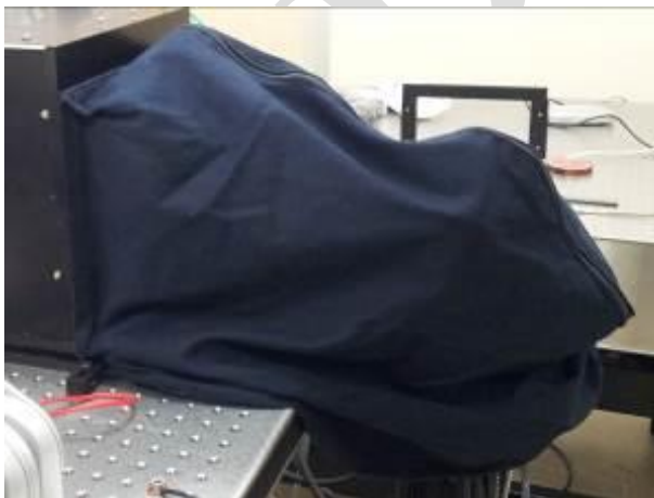
Figura 6. Image of the PnCCD fabric cover mounted on DX-LGSW.
