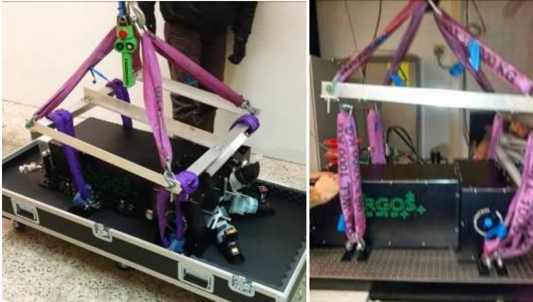
Figura 2. Pictures of the LGSW lifting frame taken during the DX-LGSW shipment.
