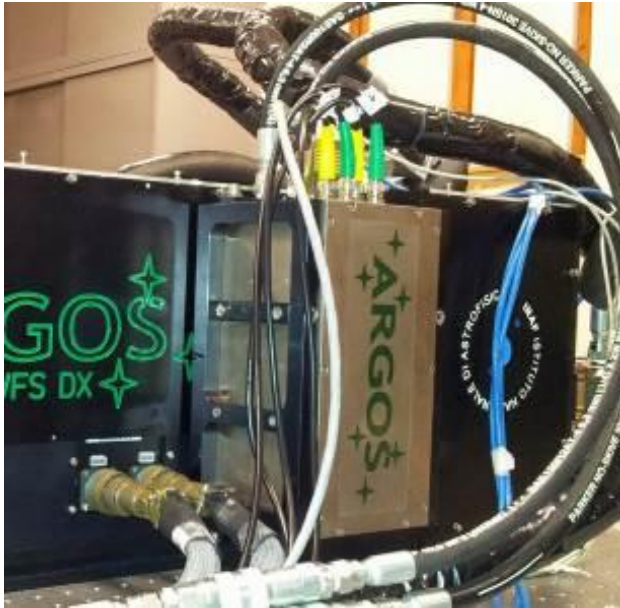
Figura 5. Pockels cell driver connected to the DX-LGSW in the lab.
