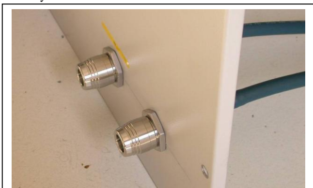
Figure 15 Detail of the Swing Arm Cabinet rear wall with cooling quick connectors. Inlet: left; outlet: right
