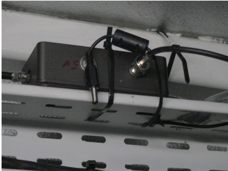
Figure 5 The trigger interface module installed in the lower-right tree-house.
