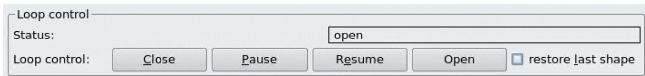
Four buttons manage the AO loop status. Because of the need of coordination between the two systems, the Close and Open buttons will send commands to both the WFS and Adaptive Secondary.
