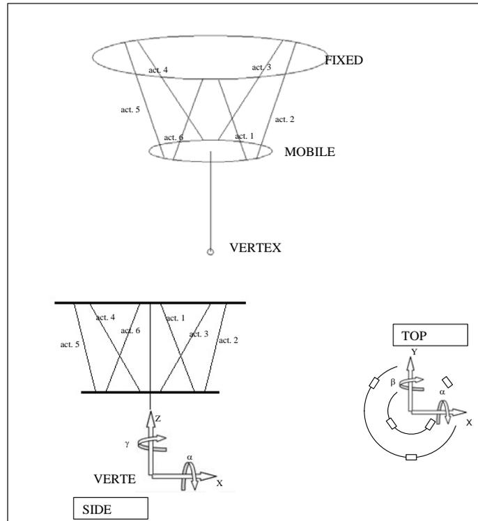
Fig. 1 Definition of Main Reference System (MRS). In the picture (from Ref. [1]) the mobile flange is in its zero position giving the M2 vertex be coincident with MRS origin O. The MRS does not move when the mobile flange moves.
