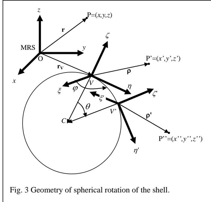
Fig. 3 Geometry of spherical rotation of the shell.
