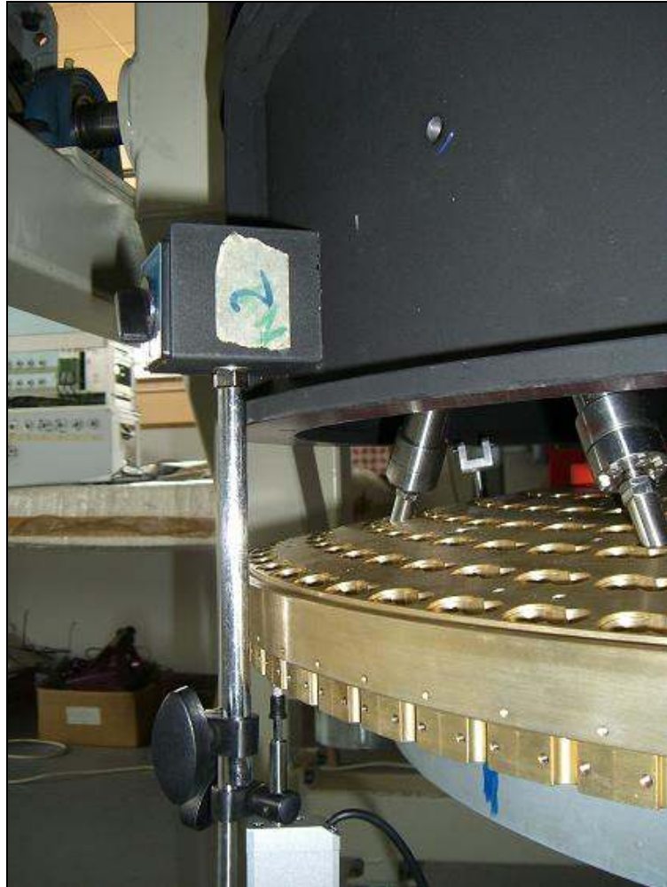
Figure 9: magnetic base mounted on the hub; the encoder is sensing the B point of the cold plate
