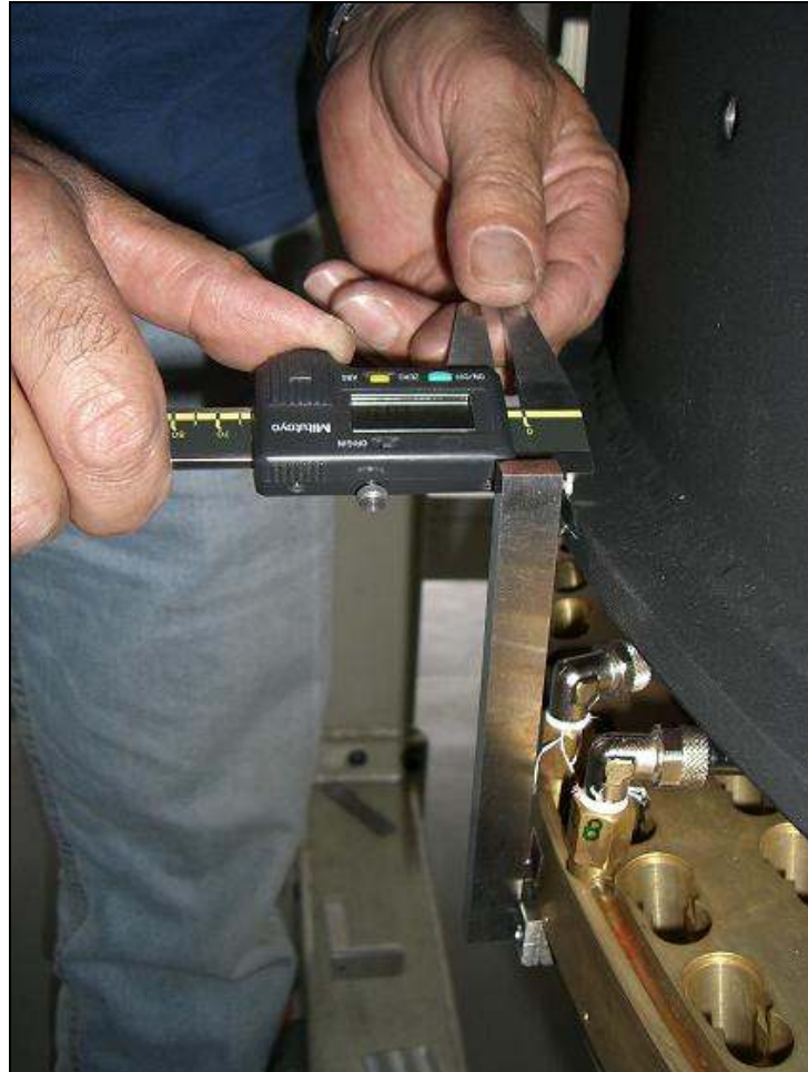
Figure 4: Measurement of the coldplate to hub radial distance.
